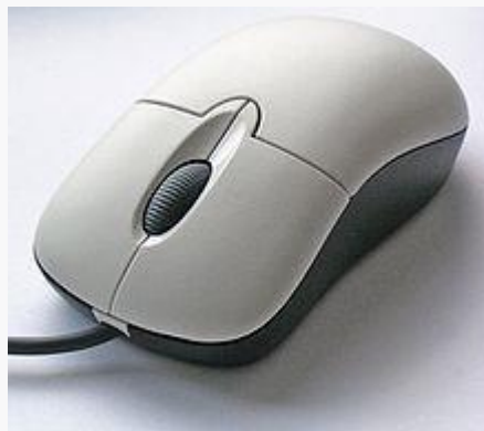
A computer mouse with the most common features: two buttons (left and right) and a scroll wheel (which also functions as a button).
