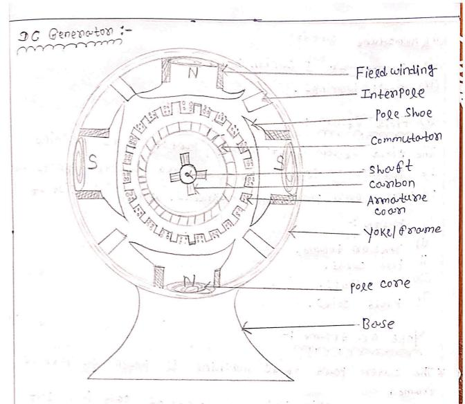
\* DC Generator is a Generator which convert machanical energy to dc voltage source.
