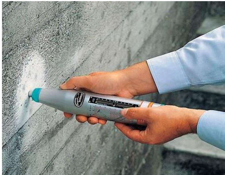
NDT test on concrete
