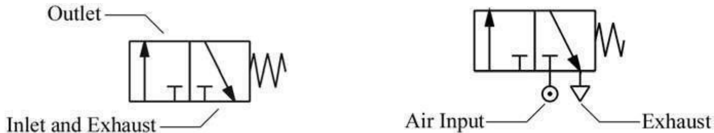
Fig173/2directionalcontrolvalve (normally closed type)
