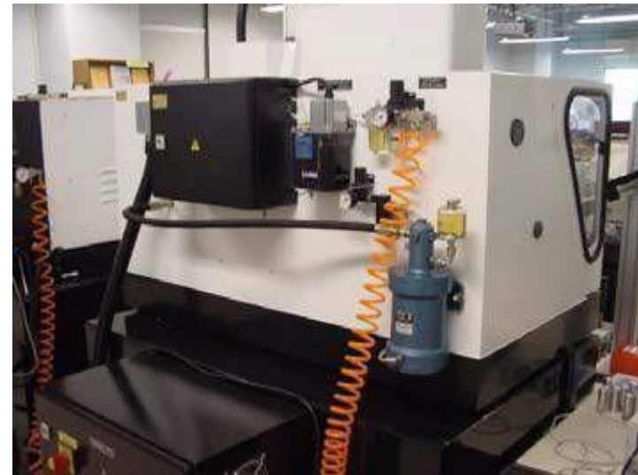
(b) Pneumatic system of an automatic machine
