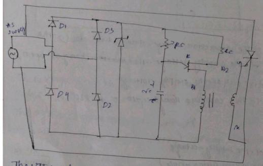
The vIt is at two layest py device with three termigals, The terminals are culted emitten (B), base -1 (B1) and base - 2 (B2).9+ consists of an nappe solicon bur withohmer cornects for the two base turnigal Asingle ptype emitten junction is formed by alloying a ptype material of the Fide of the silicen bon.
