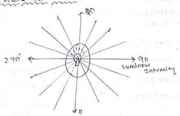
Polan curve to in which the luminous intensity is measured in ventical plane at various angle or angular Positions of a light sounces.
