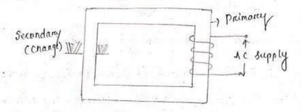
of some insulating material and primary winding connected to AC Supply.
