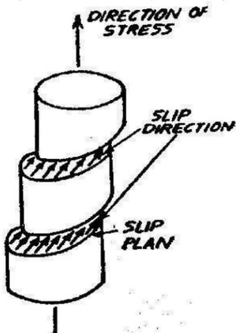
Slip is defined as the process or mechanism by which a large displacement of one part of the crystal relative to another along particular crystallographic planes takes place. There may be one or more slip planes and one or more slip directions in each crystal.
