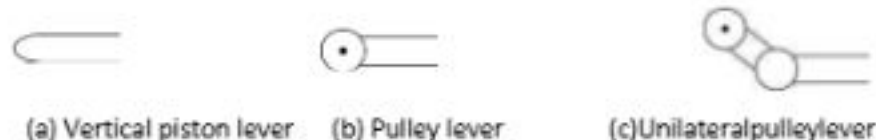
Fig. 18 Mechanically operated pneumatic components
