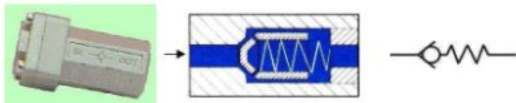
Fig.13(a)Non-return valve(b)Crosssection(c)Pneumatics symbol
