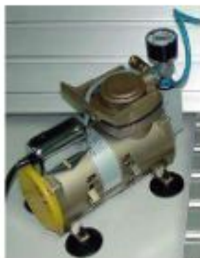
(b) Compressor used in laboratories
