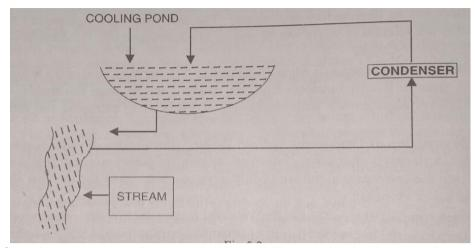
Thewaterfromthecondensersisstored intheearthlikepondswhere natural evaporation brings down the temperature. The water is recirculated again.
